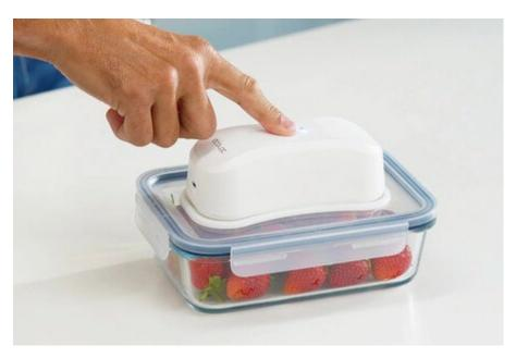
Instead, the chip leverages a physical process called cathodoluminescence to emit primarily UVC light, along with some UVA and UVB light, when excited by electrons. It's designed to initially turn on for a few minutes when food is placed in the container and then automatically turn off using a built-in timer. Users can then choose to turn it on for a few minutes each day.
